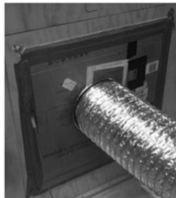
Cardboard + Fan/Flowmeter (CFF)
